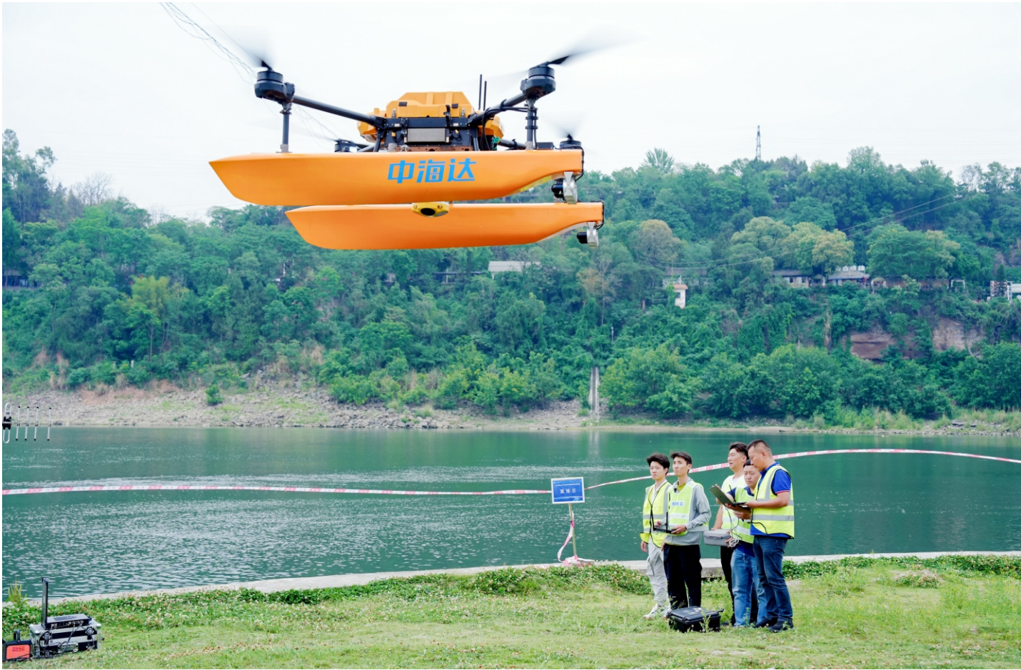
(电动两栖四轴无人机测流)
